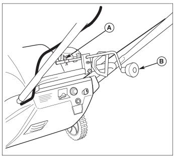
Figure 6. Discharge Chute Control Adjustment A. Cotter Pin
